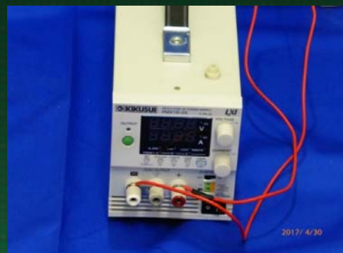
Picture 3-2 DC Power Source (Kikusui PMX 18-2A)
